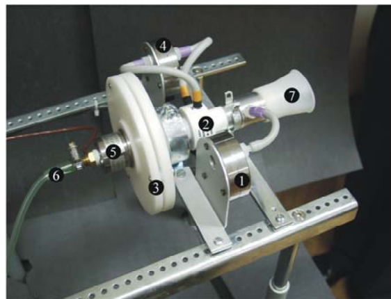
Fig. 12. The measurement station used to diagnose the respiratory system. 1 – the expiratory airflow pressure sensor, 2 – the flow measurement, 3 – the Venturi apparatus allowing to generate pressure impulses, 4 – the pressure sensor cooperating with the pneumo-tachometer, 5 – the electrical valve controlling the compressed air flow, 6 – providing compressed air, 7 – the mouthpiece.
